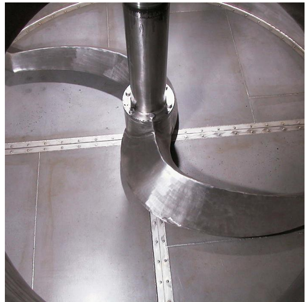
S-shaped Agitator of Nutsche Filter Dryer
